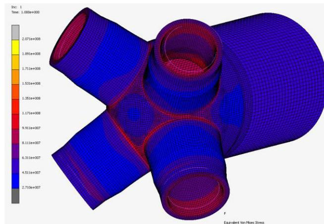
Figure 5: FEA results used for fatigue design check.
