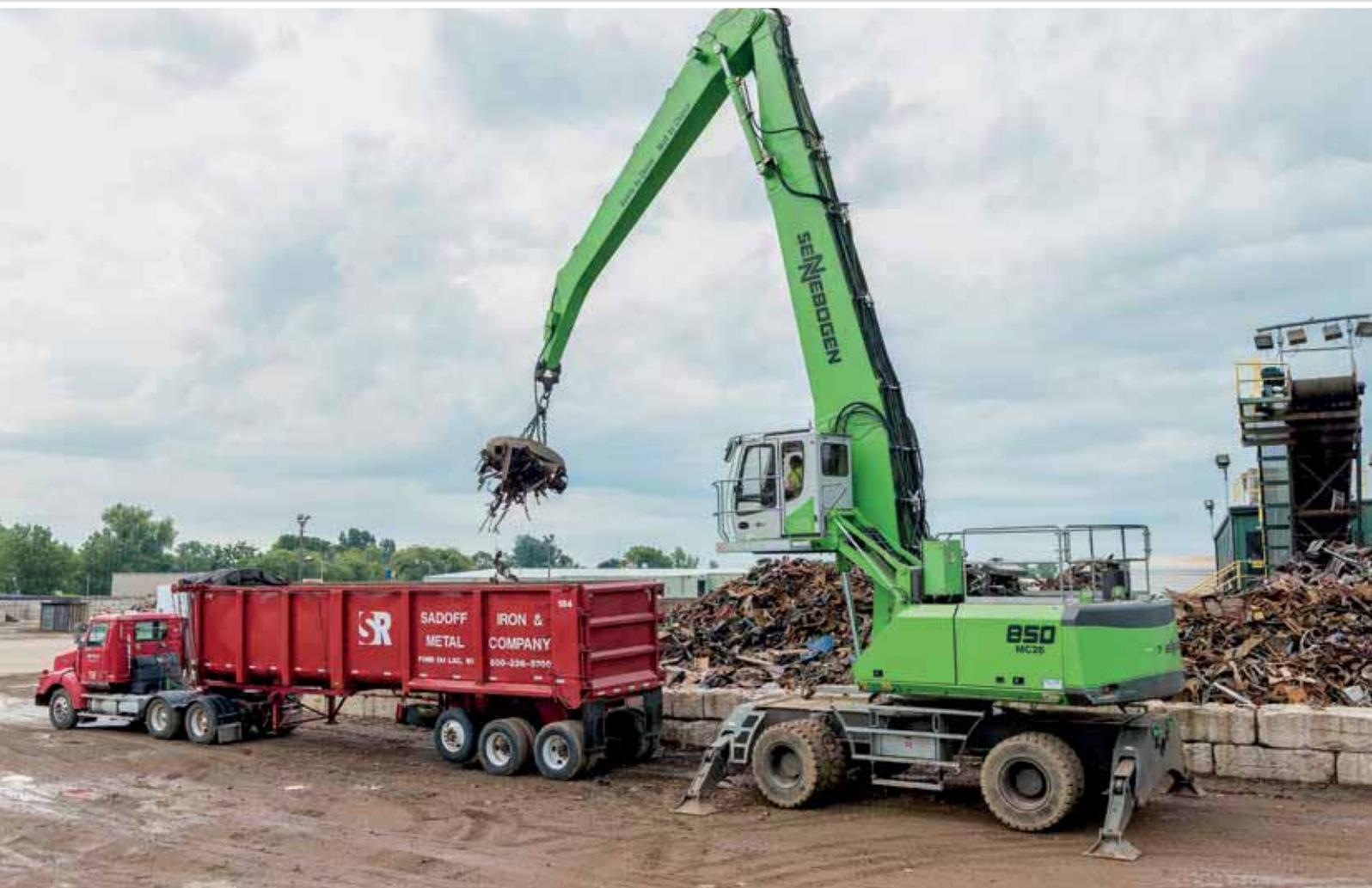
26 850 M - with magnet plate - truck loading; USA
