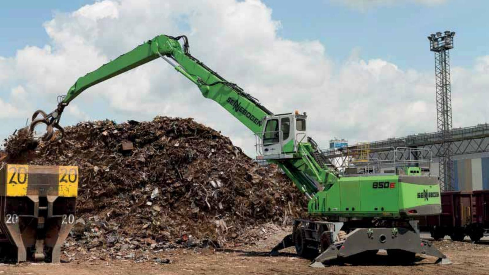
850 M - with orange peel grab - scrap handling; Austria
