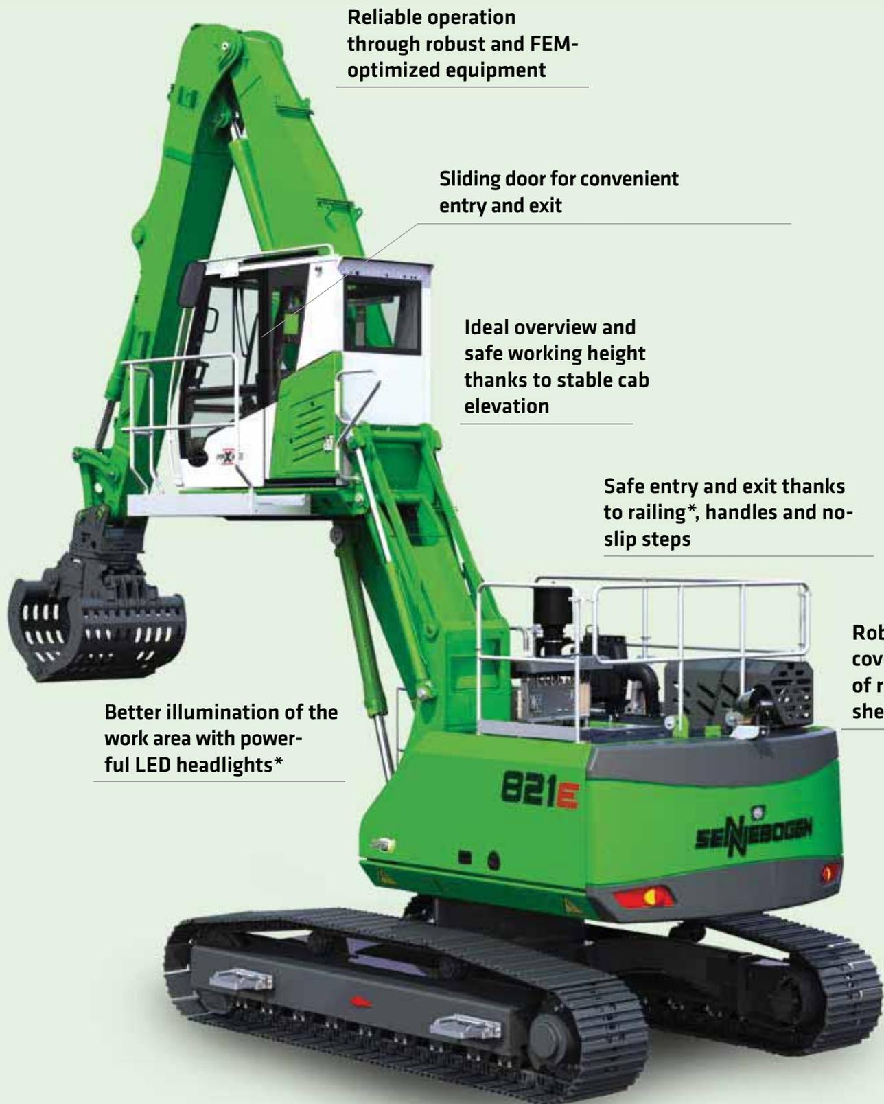
Reliable operation through robust and FEM-optimized equipment
