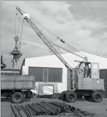
1962: Rope-driven S833 with elevated operator cab
