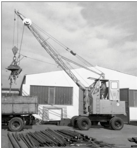
1962: rope-driven S833 with elevated operator cab
